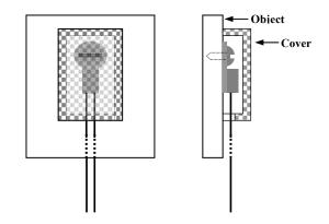
Figure 3. Using an Insulation Cover to Improve Accuracy
