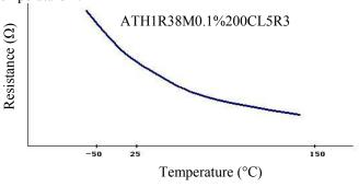
Figure 5. Resistance vs. Temperature
