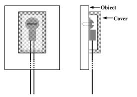
Figure 4. Using an Insulation Cover to Improve Accuracy
