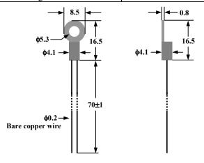
Figure 3. The Front and Side Views of ATH1R38M0.1%200CL5R3
