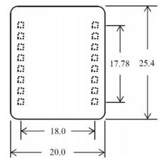
Figure 7. Top View of LDA1-CP1-D
