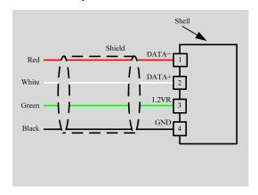
Figure 3. Connecting DAC Board to the laser Driver ATLS500MA118
