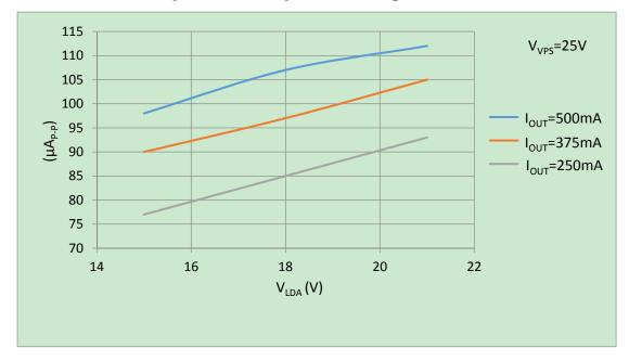
Figure 6. V<sub>LDA</sub> vs. Output Current Noise@0.1Hz~10Hz
