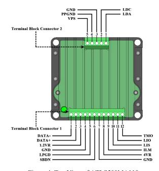
Figure 4. Top View of ATLS500MA118
