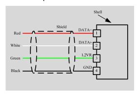
Figure 3. Connecting DAC Board to the Laser Driver ATLS2A118
