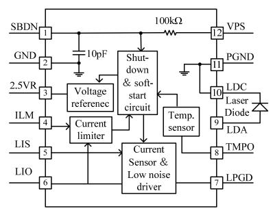
Figure 3. Block Diagram
