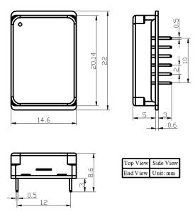
Figure 18. Dimensions of the DIP Package Controller
