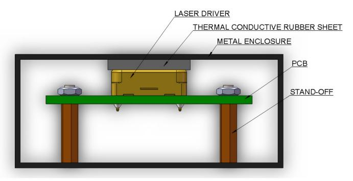
Figure 14.1 Transferring Heat with Metal Enclosure
