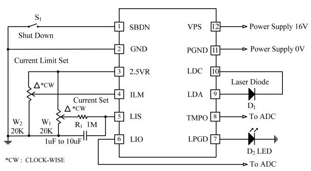
Figure 4. Typical Stand-alone CW Operation Schematic for ATLS250MA116D
