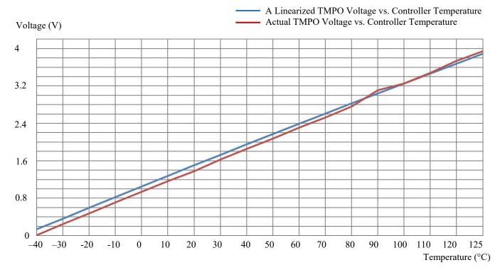
Figure 17. Controller Internal Temperature vs. TMPO Voltage
