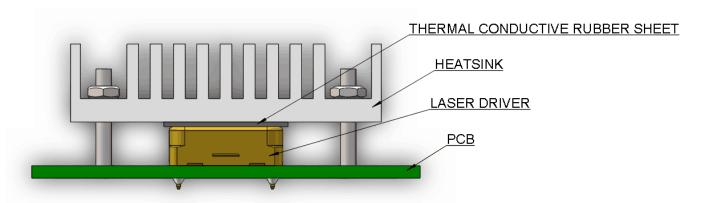
Figure 14.2 Transferring Heat with Heat Sink
