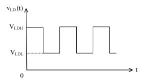
Figure 8B. Laser Diode Voltage v<sub>LD</sub>(t) Waveform
