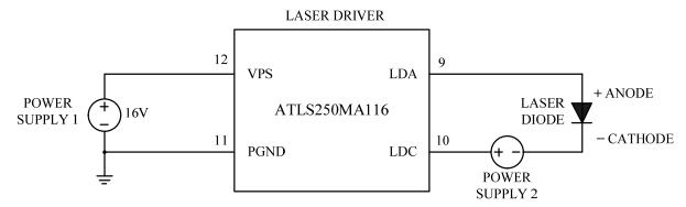
Figure 16. Driving High Voltage Laser Diodes
