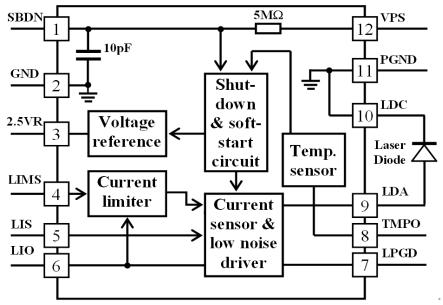
Figure 4. Block Diagram
