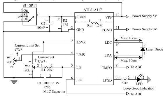
Figure 5.1. Typical Stand-alone CW Operation Schematic for ATLS1A117
