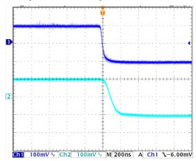
Figure 12.4. Small Signal Fall Time 200ns
