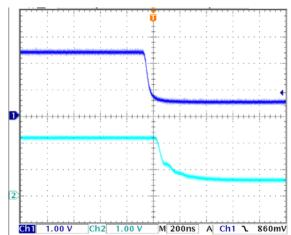
Figure 12.2. Large Signal Fall Time 220ns
