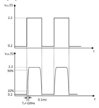
Figure 14. Large Signal Modulation
