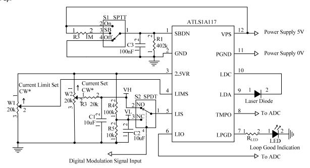
Figure 8. Low Noise Digital Modulation Circuit
