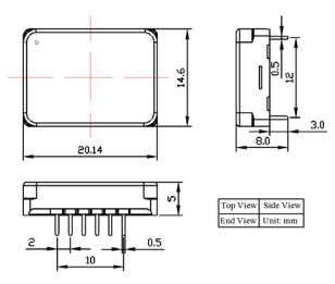
Figure 19. Dimensions of the DIP Package Controller
