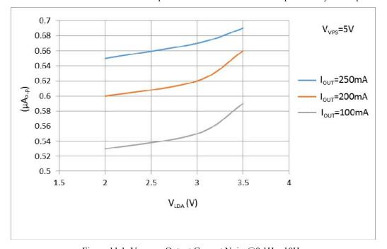
Figure 11.1. V<sub>LDA</sub> vs. Output Current Noise@0.1Hz~10Hz
