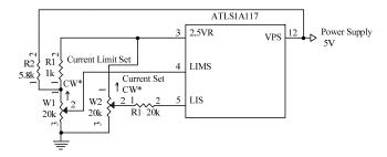
Figure 7. V<sub>LIMS</sub> setting lager than V<sub>LIS</sub>
