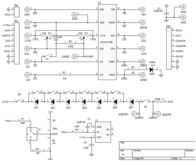
Figure 7. Schematic of ATLS100MA116DEV1.0
