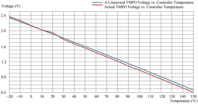
Figure 8. Controller Internal Temperature vs. TMPO Voltage
