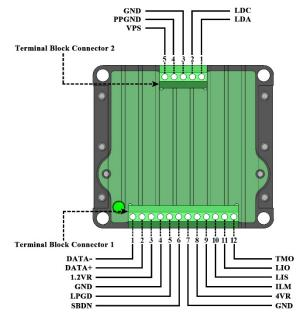
Figure 4. Top View of ATLS100MA118
