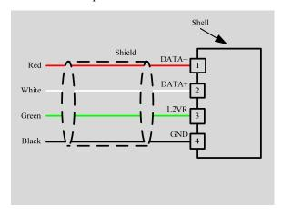
Figure 3. Connecting DAC Board to the laser Driver ATLS100MA118
