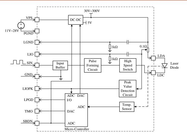
Figure 2. Block Diagram
