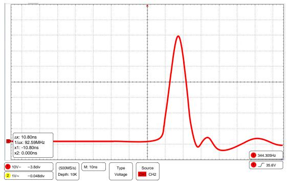
Figure 3. LDA-LDC Waveform
