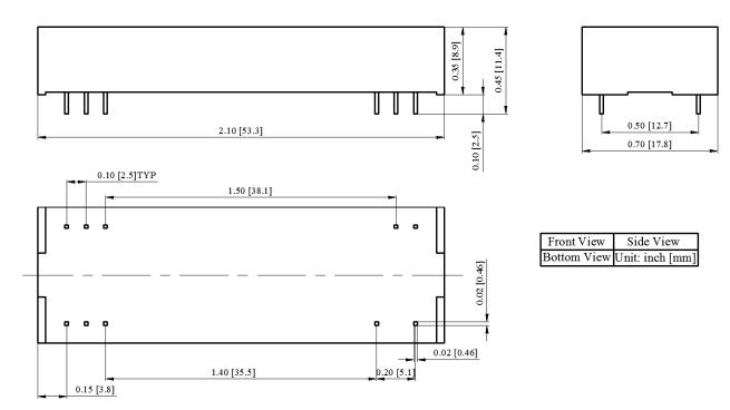
Figure 3. Dimensions of ATIA202KN DIP Package
