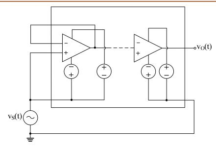
Figure 3. CMRR & CMTC Test Schematic
