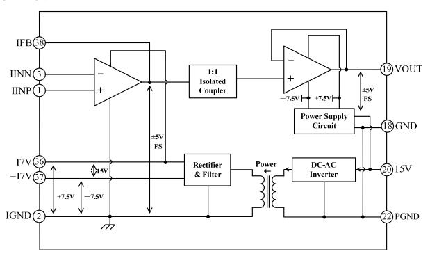
Figure 2. ATIA202KN Functional Block Diagram
